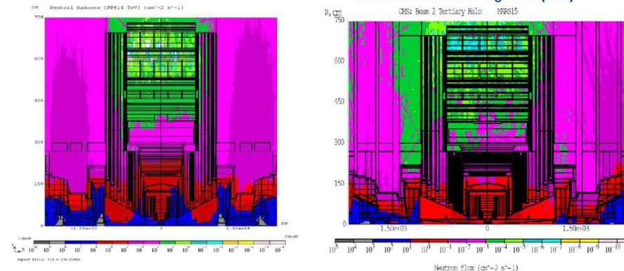
Barrel Si tracker at  $r=4$  cm:  $\Phi_n(pp) \approx 10^5 \Phi_n(MIB_{total})$ , but can differ by only a factor of 10 or so at startup conditions
