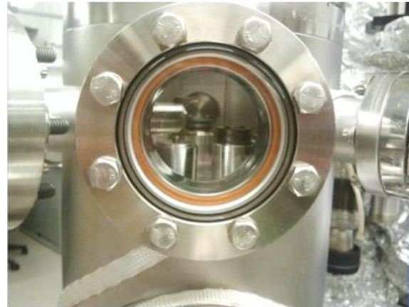
Left: Top view of the sample-introduction chamber showing all the available ports. Right: view of the sample-introduction chamber from the window that we will use to illuminate the sample for the photocurrent experiments.
