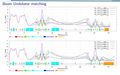
Beam transport through the U25 (top) and U90 (bottom) for 16 and 38.5 MeV beam energy and maximum and minimum field at undulators, respectively
