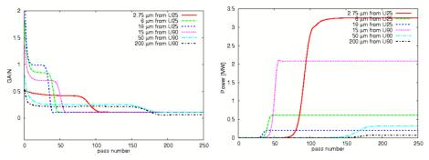
• Plots shows gain (left) and intracavity power (right) behavior versus round trips between mirrors..
