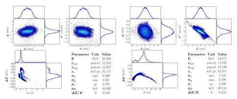
Main feature of TARLA beamline is achieving maximum beam energy with minimum bunch length. It is chromatic and almost isochronous
