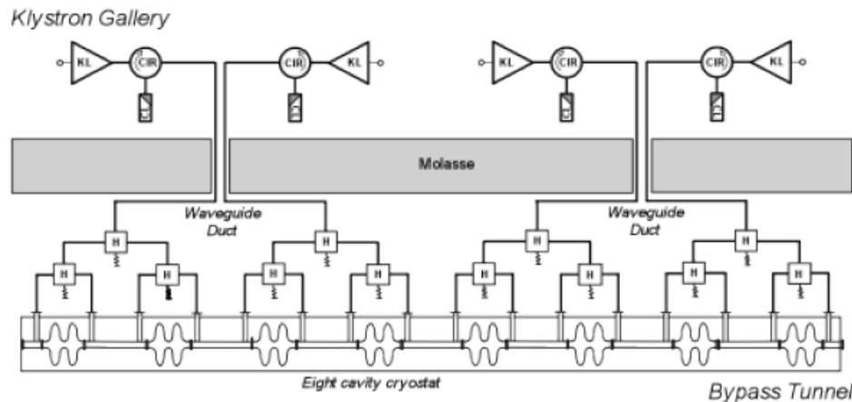
RF distribution layout for an 8-cavity cryomodule
