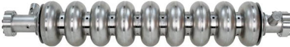
Niobium is cleaned, etched and electron beam welded
