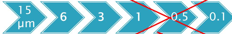
Metallography polishing in this range is not successful for flat niobium samples because regions smear or are pulled out (large-scale delamination)
