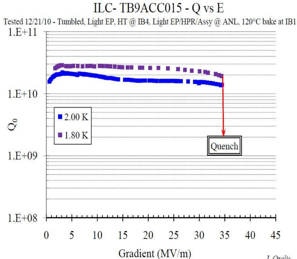
Had a large (~200micron) pit in cell 3 – previously processed and tested at JLab to 19 MV/m
