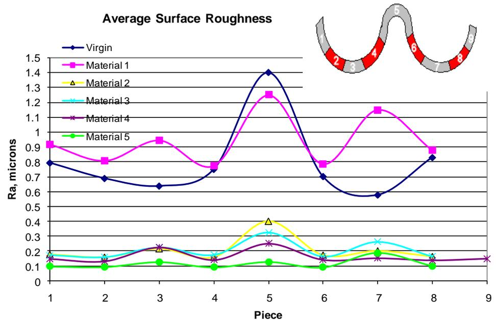
Can get Ra's on the order of 10s of nm for smaller samples of niobium using different types of media
