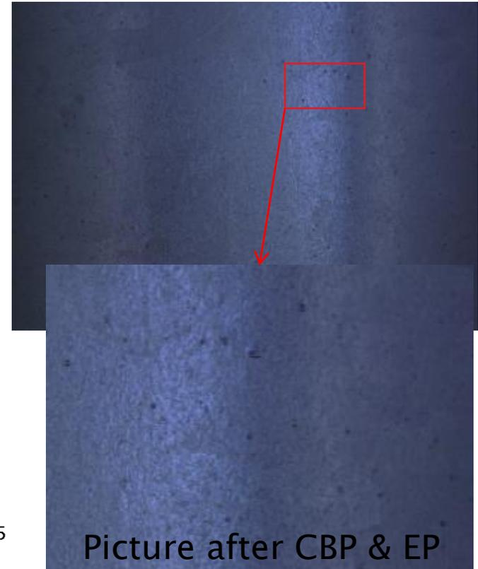
NR6 was tested after tumbling and reached as high as any of the other 6 single cell cavities from Niowave/Roark from that lot. Weld bead was successfully removed but surface shows general pitting after processing. Apparent porosity in material.
