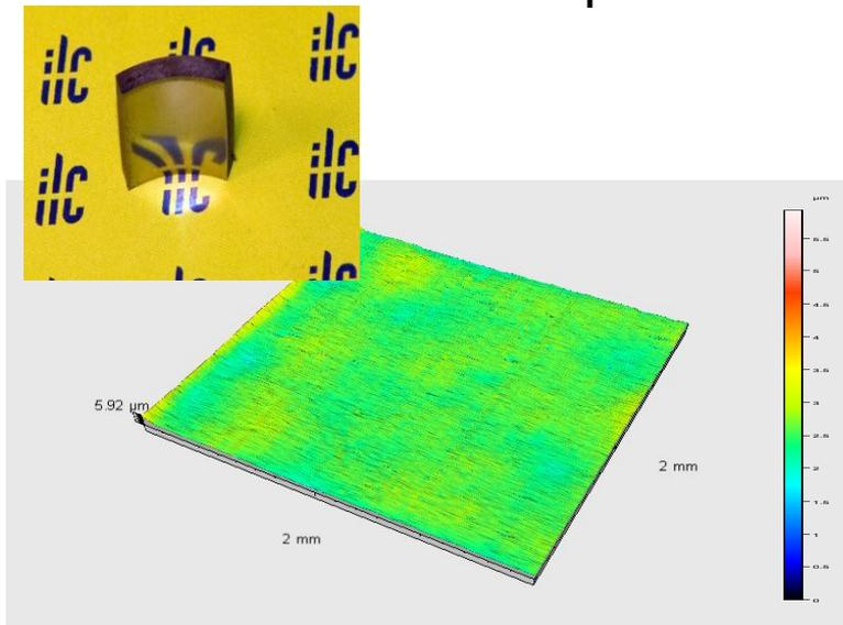
Ra = 0.00226  $\mu\text{m}$  +/- 0.000171  $\mu\text{m}$
