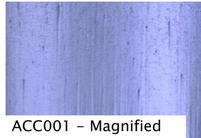
First polishing step was 5 hours instead of 12, leaving **embedded media** in the cavity. May explain drop in accelerating gradient. Quality factor did increase substantially.
