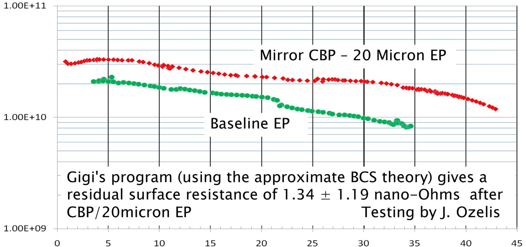
Cavity tested many times after baseline EP processing and reprocessing techniques. Best baseline results shown. Cavity improved greatly after CBP.
