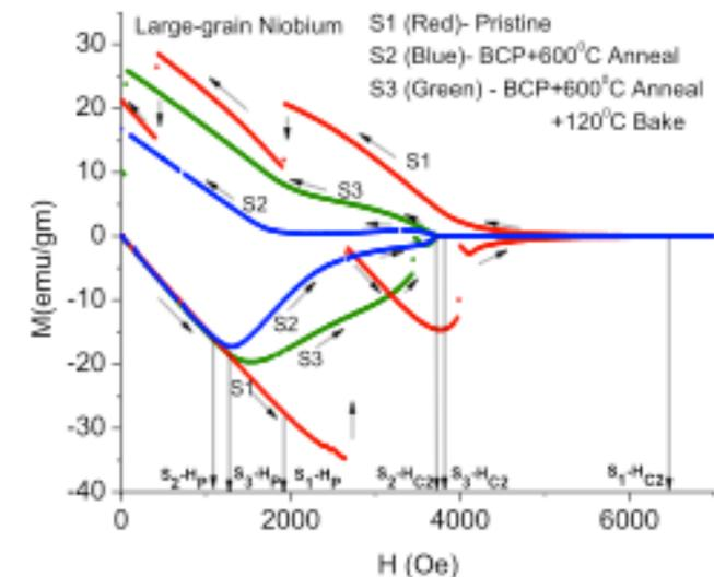
Figure 5. Isothermal  $M-H$  plots of LG-Nb samples starting from the zero field cooled state at 2 K.
