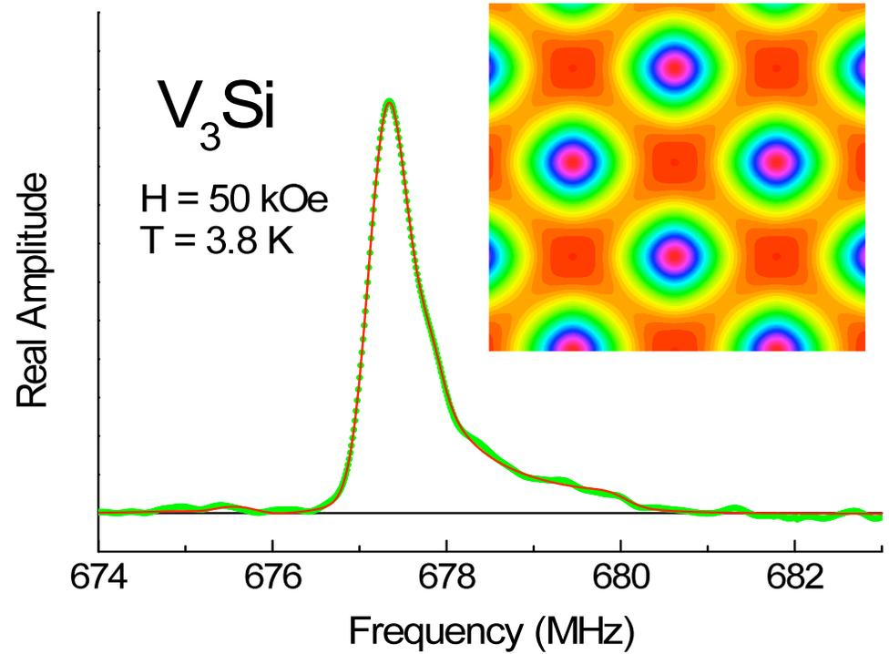
**Asymmetry spectrum plotted in a rotating reference frame**
