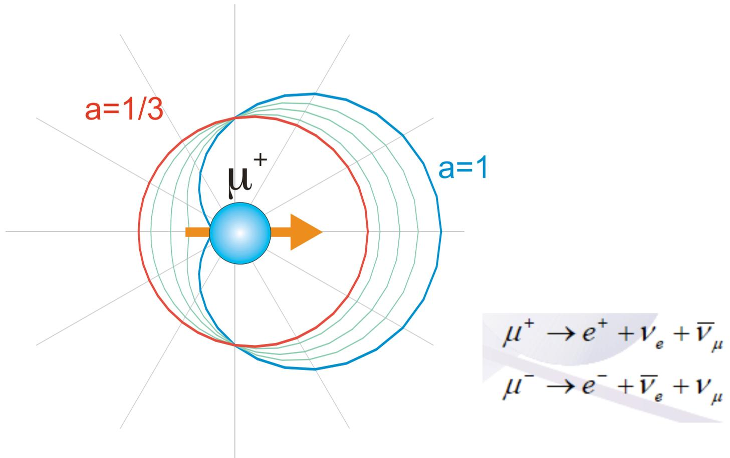
Angular distribution of positrons from the  $\mu^+$ -decay. The asymmetry is  $a = 1/3$  when all positron energies are sampled with equal probability.
