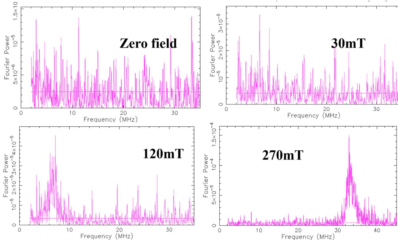
Fast Fourier transforms for sample H1 at 2.3K and respectively field levels: zero, 30mT, 120mT (peak of flux appearing at  $\sim 50$ mT), 270mT (peak of flux  $\sim 260$ mT)
