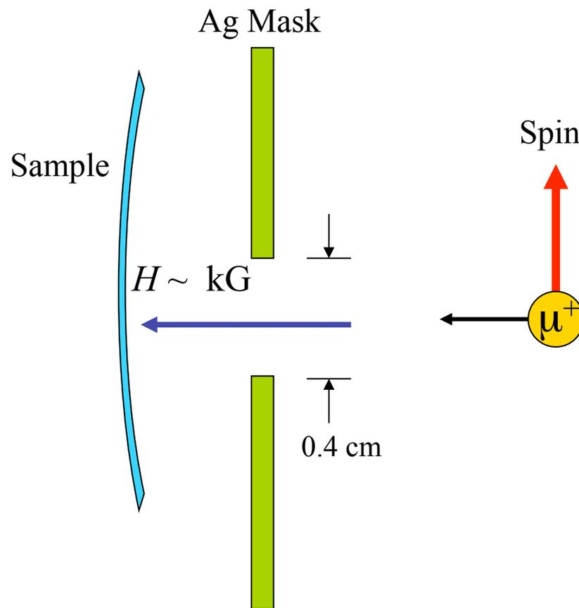
Muon stopping depth  $\sim 300\mu\text{m}$
