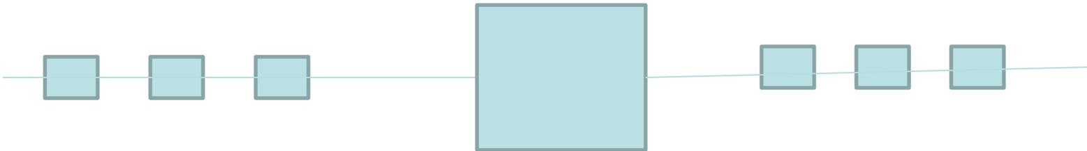
3 + 3 BPMs; define and verify straight line before and after quad under test (QUT)
