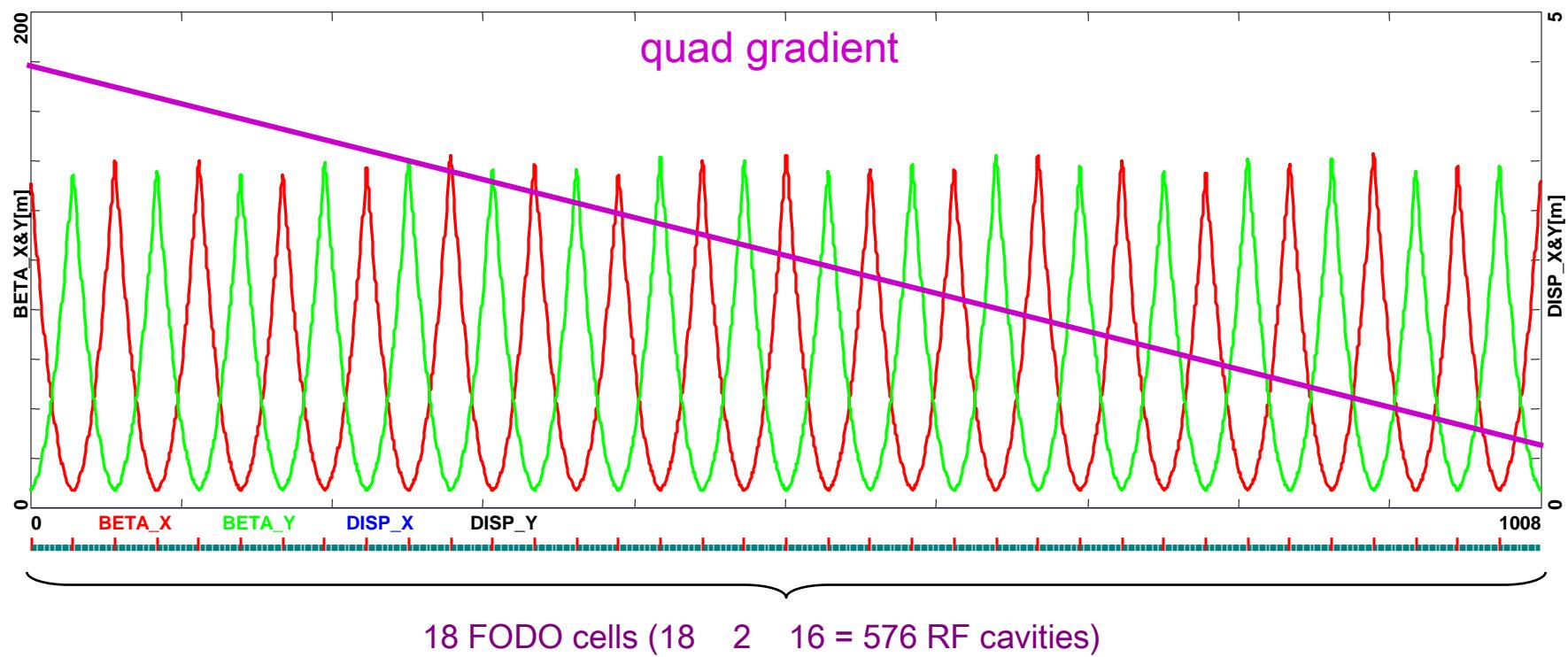
Linac 2 multi-pass optics with ER – mirror symmetric to Linac 1
