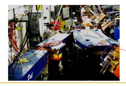
Proton Storage Ring (PSR) at Los Alamos LANSCE facility. Dipole on the right has a bending angle of 36 degrees, path length of 2.54948 m and sagitta of 23.83 cm.
