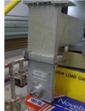
“symmetric” adapter only good for TE 10
