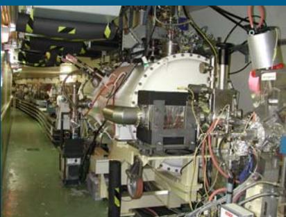
Supraconducting radio frequency cavity: made of Copper + Niobium
