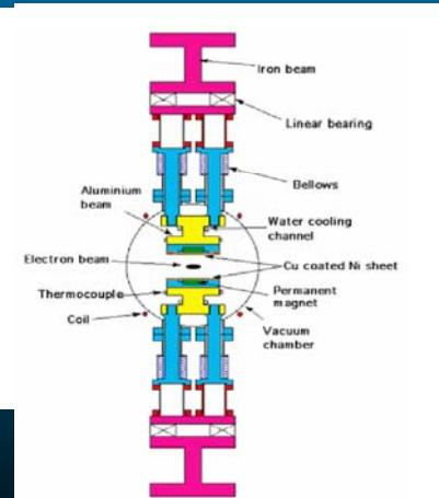
Magnetic blocks in the vacuum with an operating magnetic gap of 4 – 6 mm
