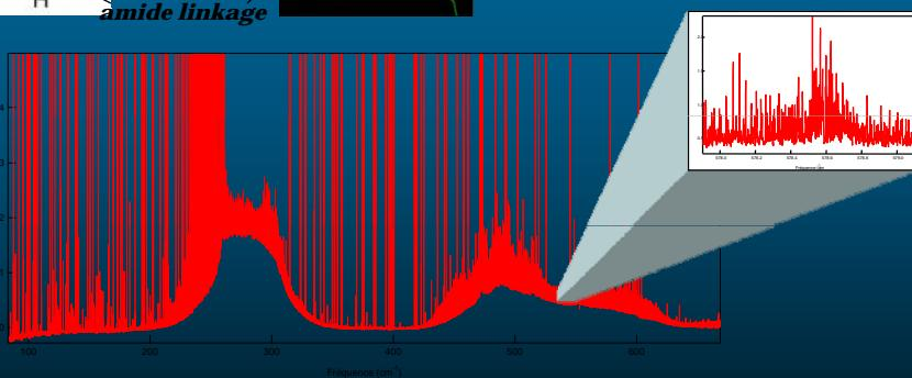
The absorption spectrum is fully resolved thanks to the combination of the high resolution interferometer with a 200 m path cell at low pressure.
