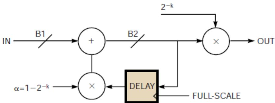
$$H(z) = \frac{N(z)}{D(z)} = \frac{b_0 + b_1 z^{-1} + b_2 z^{-2} + \dots + b_M z^{-M}}{1 + a_1 z^{-1} + a_2 z^{-2} + \dots + a_N z^{-N}}$$
