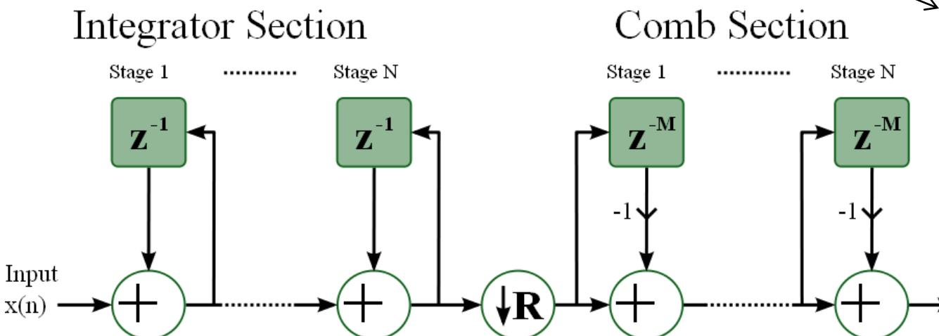
Decimating cascaded integrator-comb (CIC) filter;  $N$  stages,  $R$  decimation,  $M$  delays
