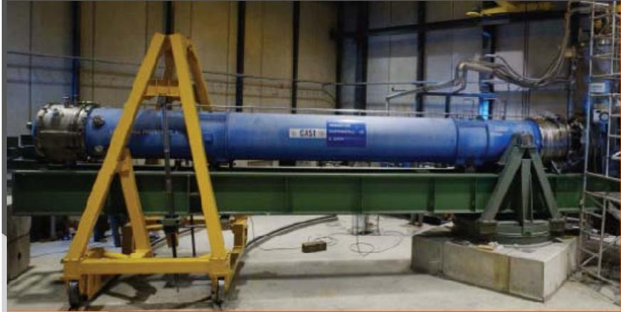
Uses LHC prototype dipole, looks for axions from the sun regenerating photons in the x-ray region. K. Zioutas *et al.*, PRL 94, 121301 (2005)
