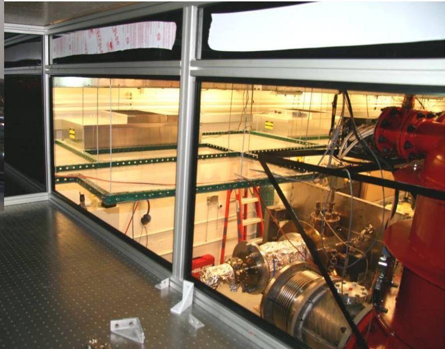
**A new transfer system for moving the SF6 from the gun and HVPS to the storage bag was designed and built with pneumatic valves and electronic controls**
