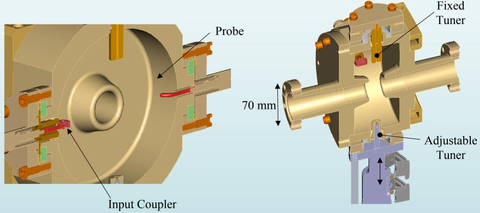
FZ Rossendorf design, modified for ERLP, manufactured by Vacuum Generators (UK)
