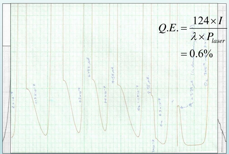
After cathode re-activation on 30/08/06, the gun exhibited huge out-gassing during HV conditioning.
