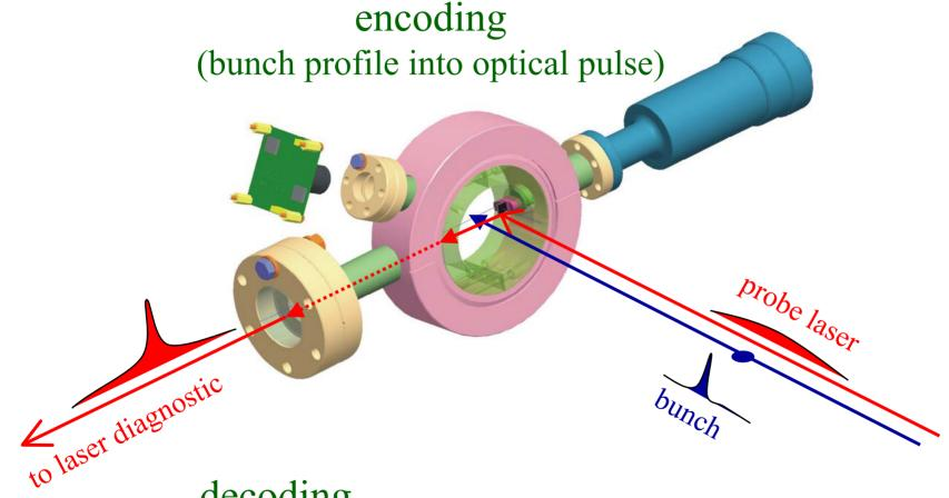
decoding (optical pulse into profile measurement)
