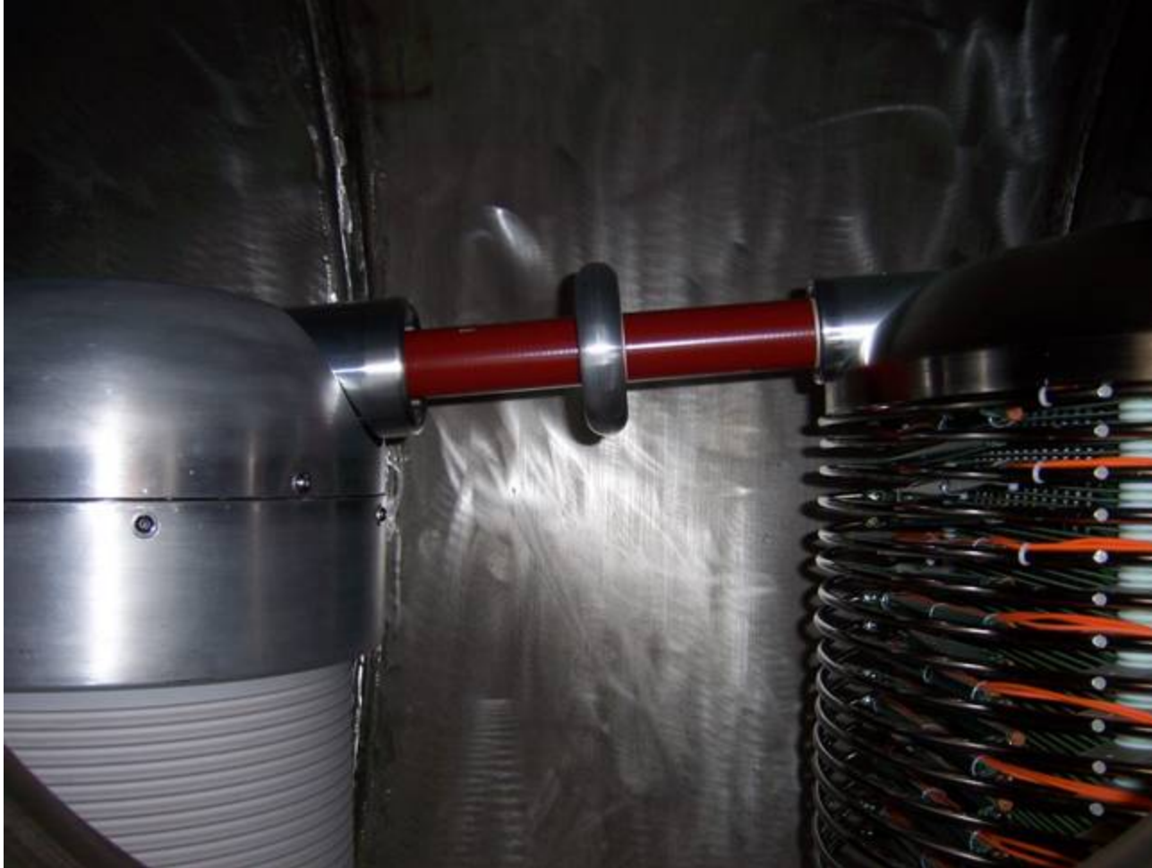
Floating ammeter mounted on the processing resistor
