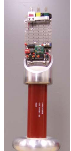
Floating ammeter mounted on the processing resistor
