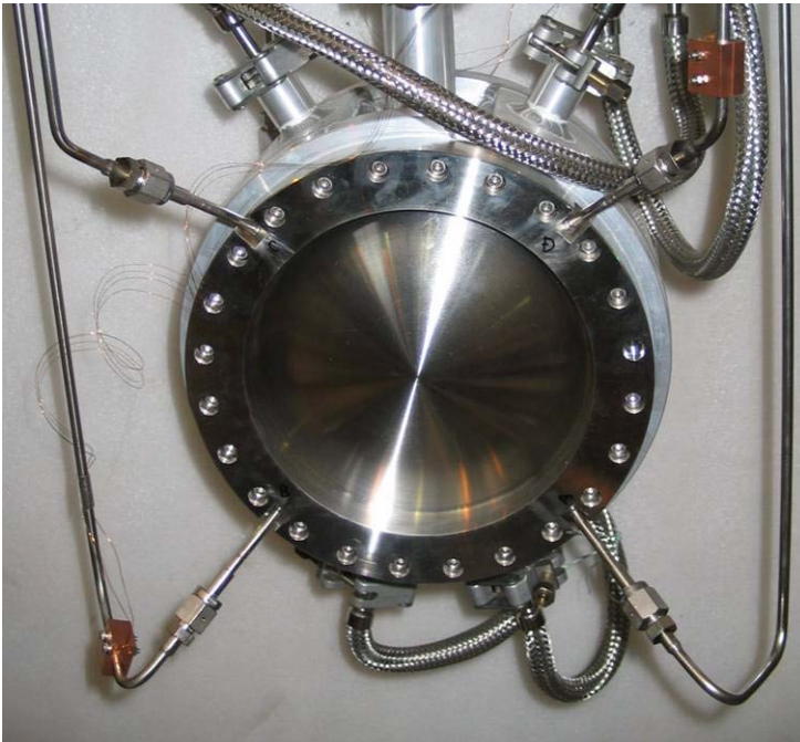
Prototype high-power LH 2 absorber (MuCool)
