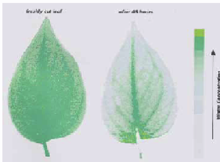
THz images of a fresh leaf and of the same leaf after 48 hrs
