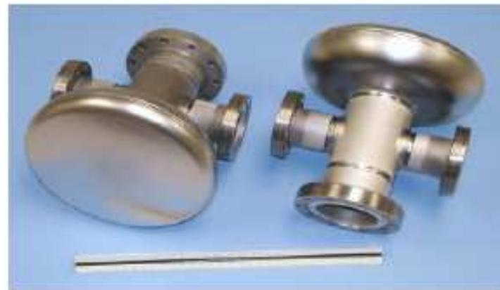
Figure 4: Photograph of  $\frac{1}{2}$  cell Nb cavity
