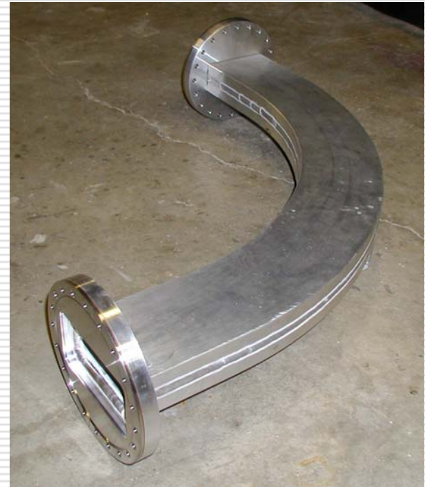
Vacuum chamber in dipoles made of aluminum with 8" Al-SS flanges
