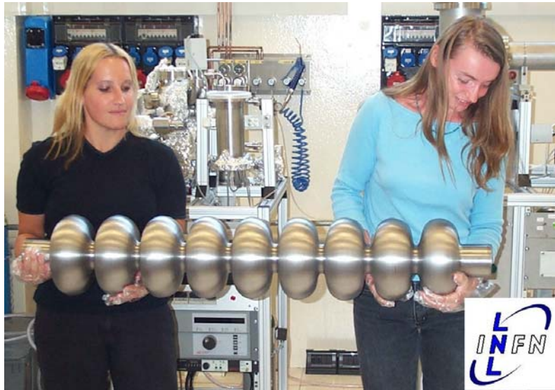
First spun 9-cell cavity
