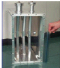
4 gap ladder, 352 MHz, \beta=0.12 INFN-LNL
