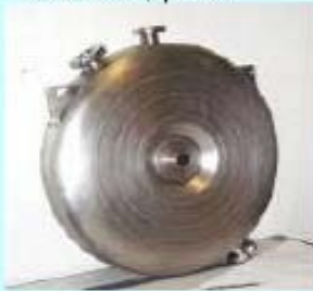
1 gap reentrant- LNL 352 MHz, \beta > 0.1
