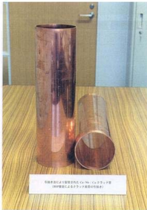
Cu-Nb-Cu Sandwiched Tubes (KEK)
