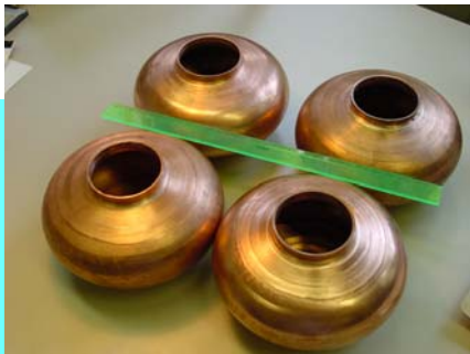
Cu-Nb-Cu Sandwiched Tubes (KEK)
