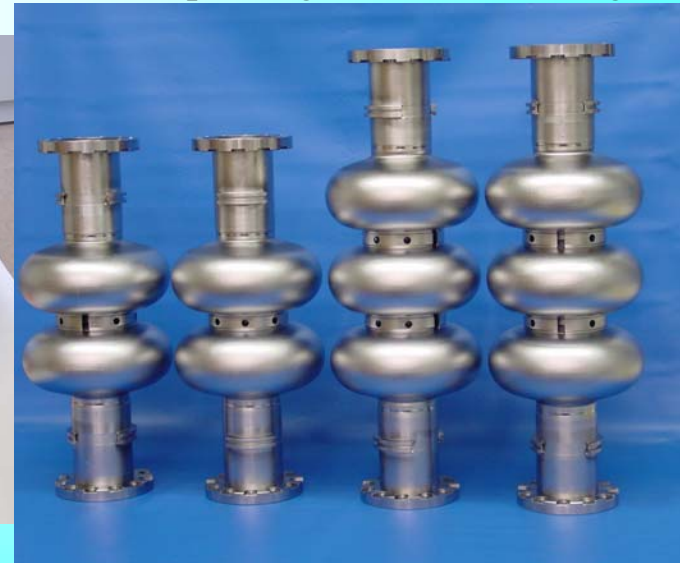
Two and three cell cavities hydroformed at DESY
