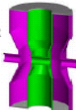
322 MHz, \beta=0.28 HWR MSU for RIA
