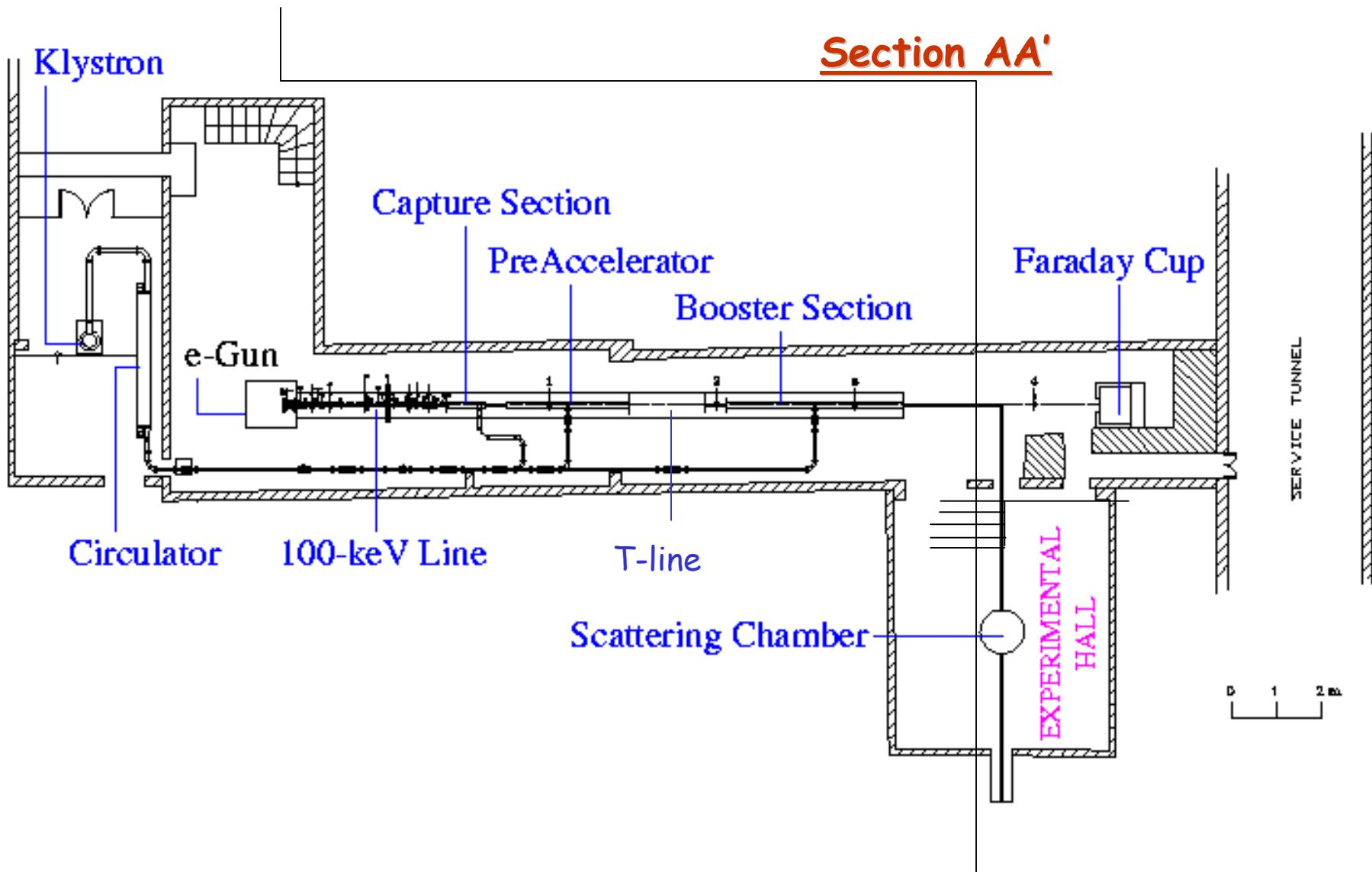
CROSS SECTION PP' OF ACCELERATOR TUNNEL & EXPERIMENTAL HALL
