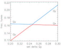
Closest tune approach dQ=0.001 after correction with skew quads
