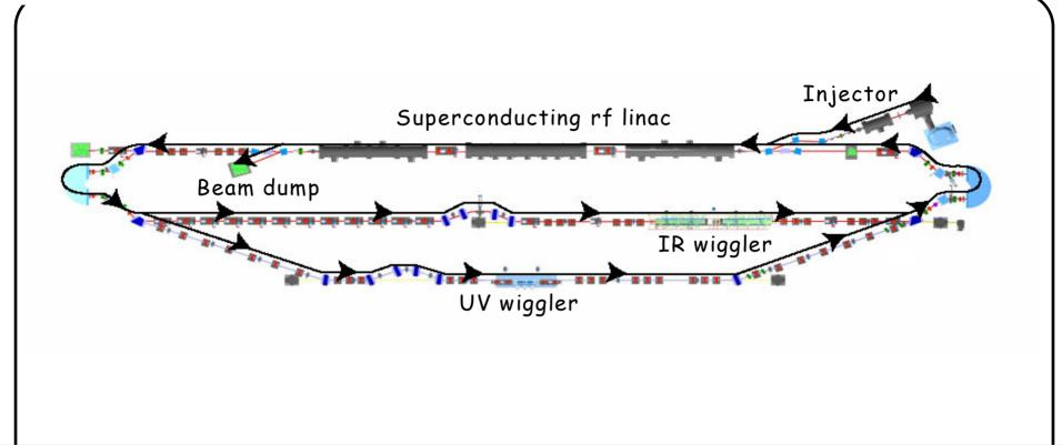
Achieved 8.5 kW CW IR power on June 24, 2004! Energy recovered up to 5mA at 145 MeV, up to 9mA at 88 MeV
