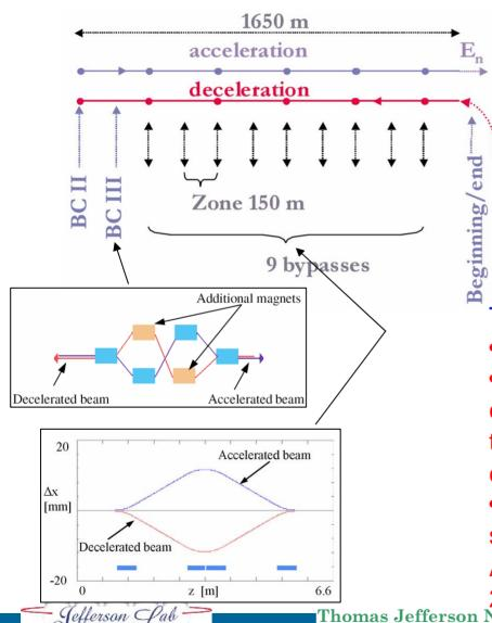
At a 1 MHz rep rate there are 6 bunches in the ERL at a given time, thus 12 collision locations separated by 150 meters.
