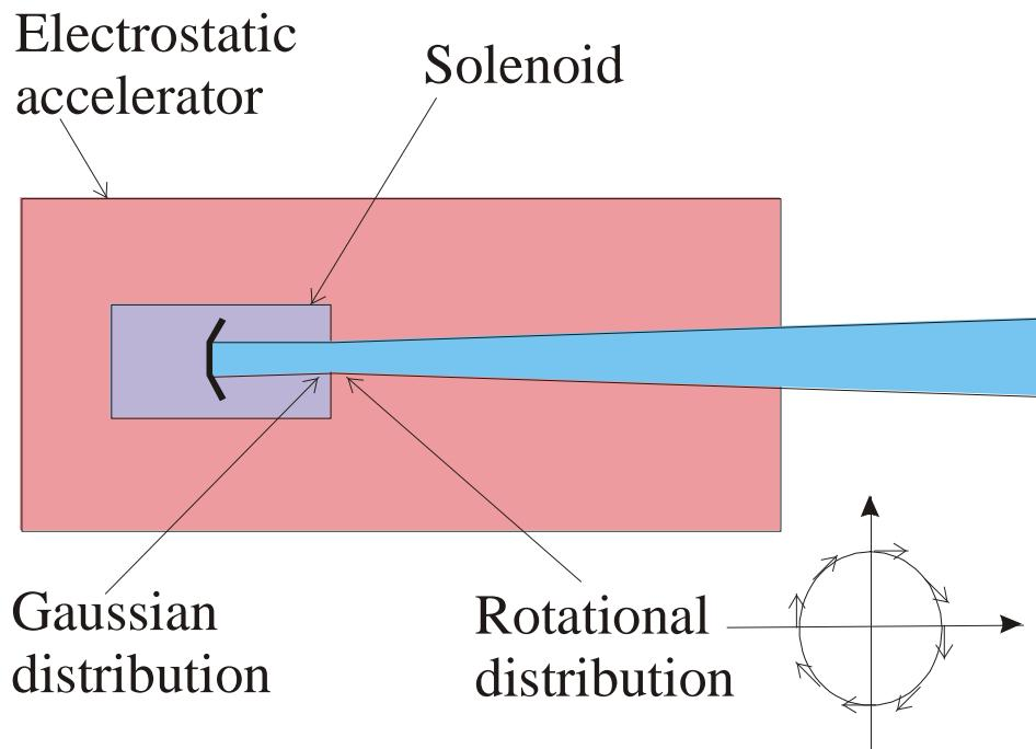
The electron beam distribution is axially symmetric, and uncoupled at the cathode:
