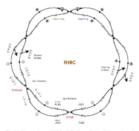
Fig. 5.1. Schematic layout of RHIC at BNL. The two Siberian Snakes per ring and their snake axes are shown.
