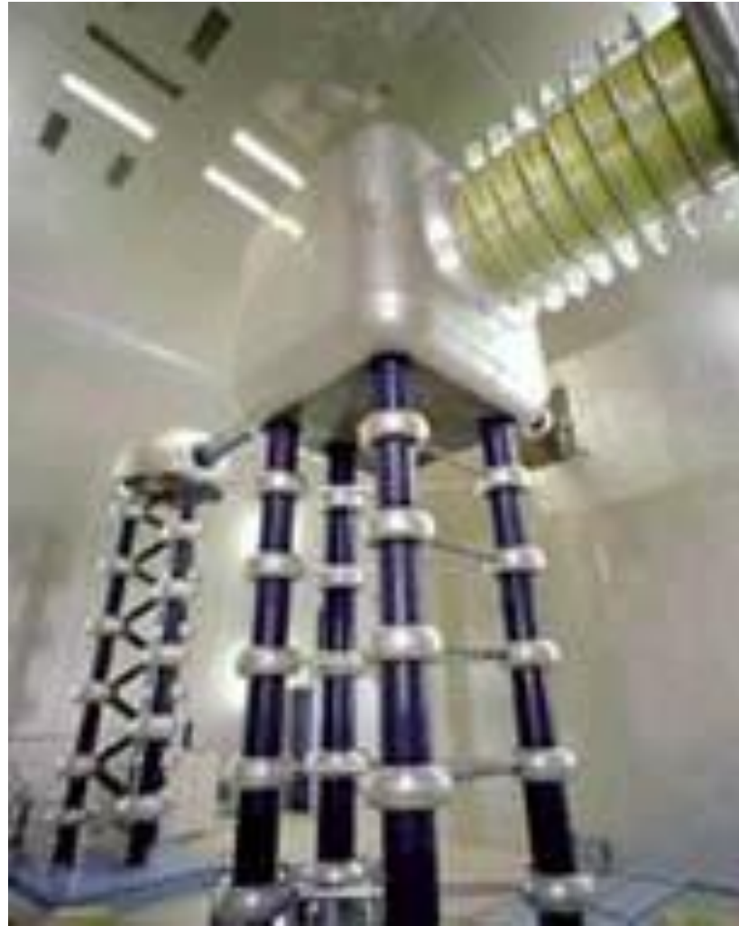
Proton Source at Fermilab, Beam Energy 750 keV
