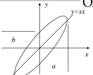
where *s* is a slope parameter, *a* is the maximum extent in the *x*-direction, and the *y*-intercept occurs at  $\pm b$ , and again  $\varepsilon$  is the area of the ellipse divided by  $\pi$
