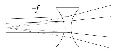
Thin Focusing Lens (limiting case when argument goes to zero!)
