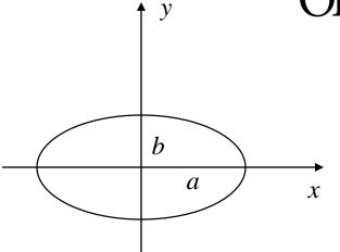
In beam optics, the equations for ellipses are normalized (by multiplication of the ellipse equation by ab) so that the area of the ellipse divided by  $\pi$  appears on the RHS of the defining equation. For a general ellipse
