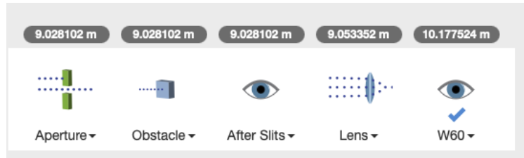
Figure 24. Young's double slit layout in SRW Sirepo. The layout consists of an aperture and obstacle that create a double slit, the drift after the slit, a lens, and watchpoint (W60).
