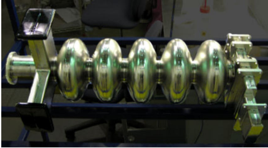
FIG. 1.2: A CEBAF 5-cell cavity with a waveguide higher-order mode coupler (left) and fundamental power coupler (right).
