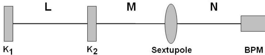
FIG. 13. A simple model of beamline elements for demonstrating how two distinct frequencies of a simultaneously modulated electron beam will mix due to the non-linear fields of a sextupole.
