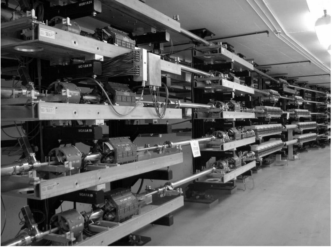
FIG. 5. A photograph showing stacks of magnet assemblies in the East Arc. The order of elements is sextupole, BPM, quadrupole and corrector (Photo from JLAB archive).
