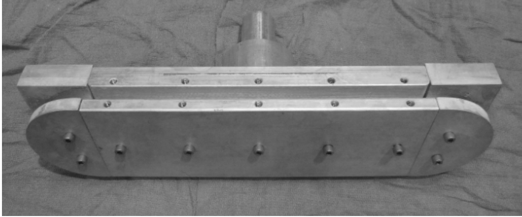
FIG. 20. A picture of the winding fixture that was used to make the coils.
