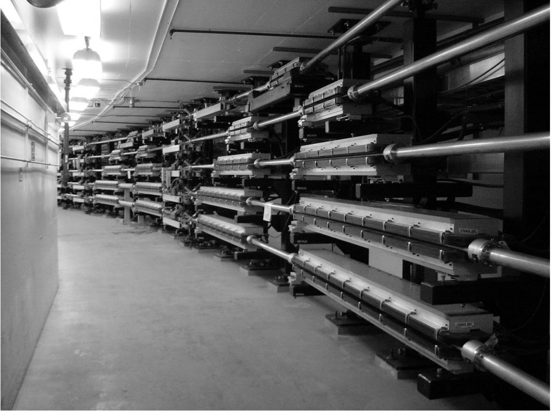
FIG. 4. A photograph of a section of the East Arc. The lowest energy Arc 1 beamline is at the top with Arcs 3,5,7 and 9 stacked below (Photo from JLAB archive).
