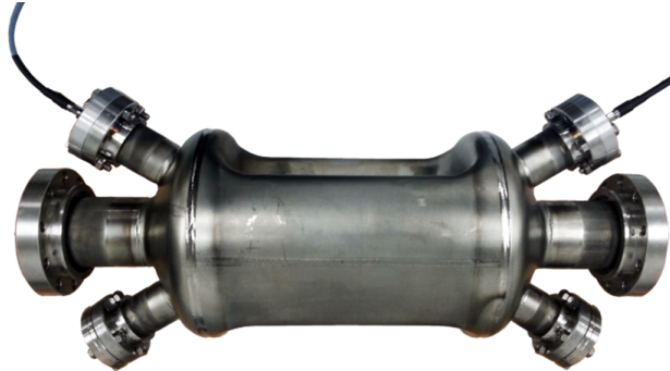
FIG. 21: Prototype of a 750 MHz rf-dipole crab cavity for MEIC.
