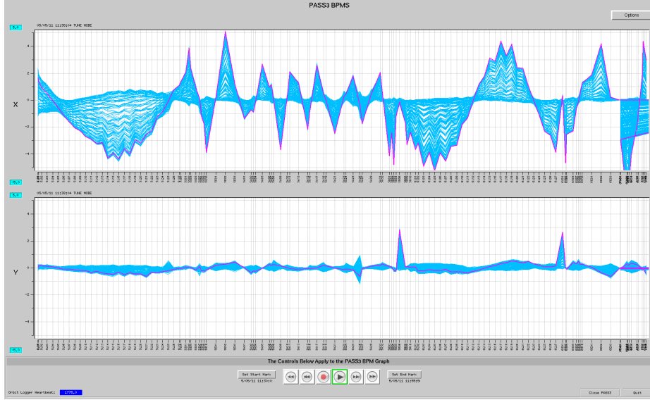
Figure 4.2: Overlaid Trajectories for 3 Pass CEBAF Machine
