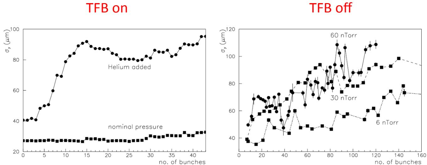
Figure 1: *RMS vertical beam size versus the number of bunches at a current of 0.5 mA/bunch: (left) for nominal and elevated pressure conditions, TFB on; (right) for three different values of the average helium pressure, TFB off.*
