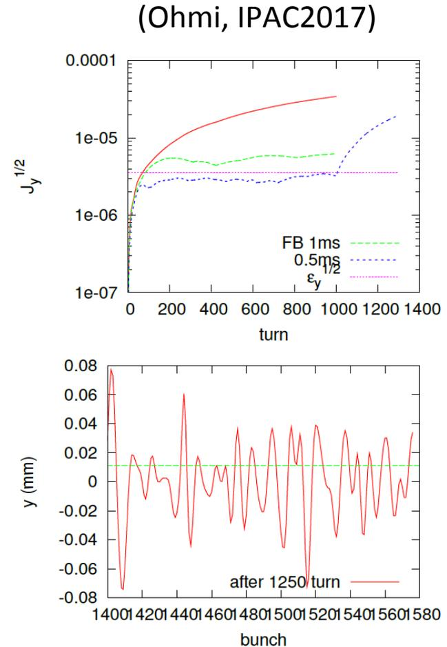
Figure 5: Ion instability in the experimental condition,  $N_b$  1576, 3 bucket spacing,  $I = 500$  mA, 100 nPa.
