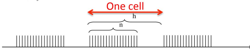
**Figure 1.** An illustration of the bunch train that shows a maximum possible  $h$  bunches out of which  $n$  bunches are filled with electrons and  $h - n$  bunches are empty.
