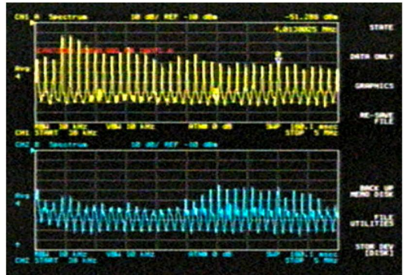
Figure 7: Transverse spectra of the HER with 16-bucket gap (34 ns). Top trace (yellow) is horizontal; bottom trace (blue), vertical motion. The frequency range is from 20 kHz to 5 MHz and the vertical scale is 10 dB/div in both spectra.
