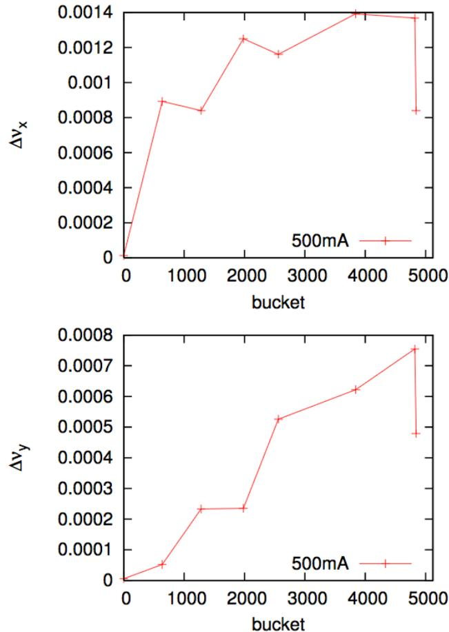
Figure 3: Horizontal (top) and vertical (bottom) tune shift along the bunch train.
