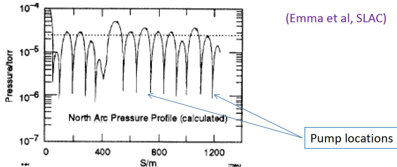
Figure 2: Pressure profile in the SLC north arc calculated according to [5]. The dips are the pump locations. The circles indicate newly installed vacuum gauges.
