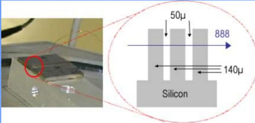
The gap between the crystal lamellae are reduced to less than the coherence length of 350 μm on ID 28.
