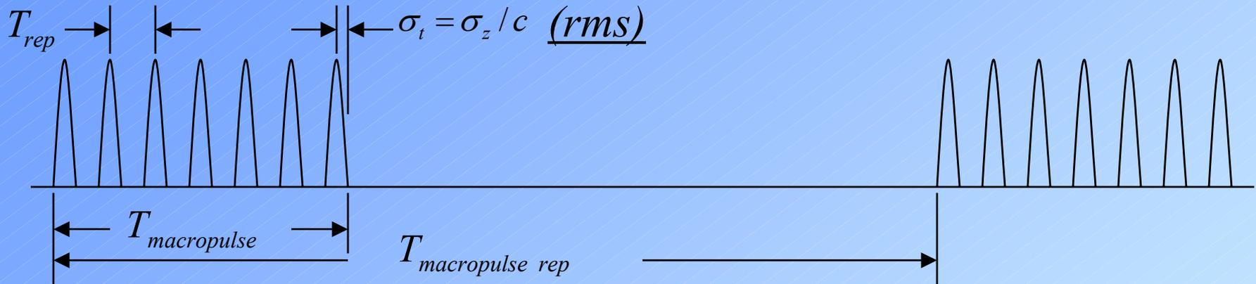
**Puls pattern is ideal for pump & probe experiments**
