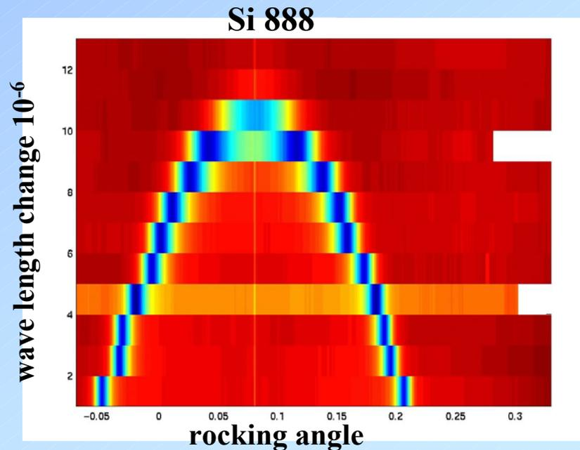
**In reality the wave fields of all 8 reflections are expected to interact with each other, i. e. they exchange energy in a complex way**
