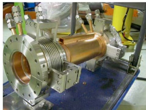
FIG. 4. Universal bellow chamber for a movable mask of KEBK LER.
