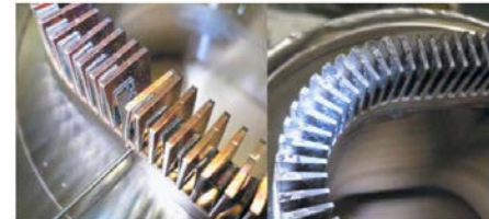
FIG. 7. Damage of teeth of the Comb-Ver.1. The teeth were slightly bent in order to check between them.
