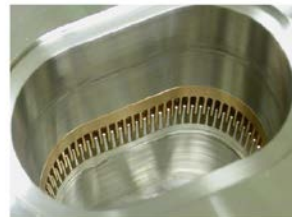
Figure 1: Racetrack bellows chamber with comb-type RF shield.
