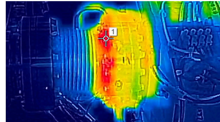
[2] Local overheating image of flange joint at NSLS-II A. Blednykh, et., al., IPAC2019, TUPGW082
