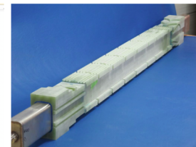
G-11 Structural beam with machined channels for CIC turns
