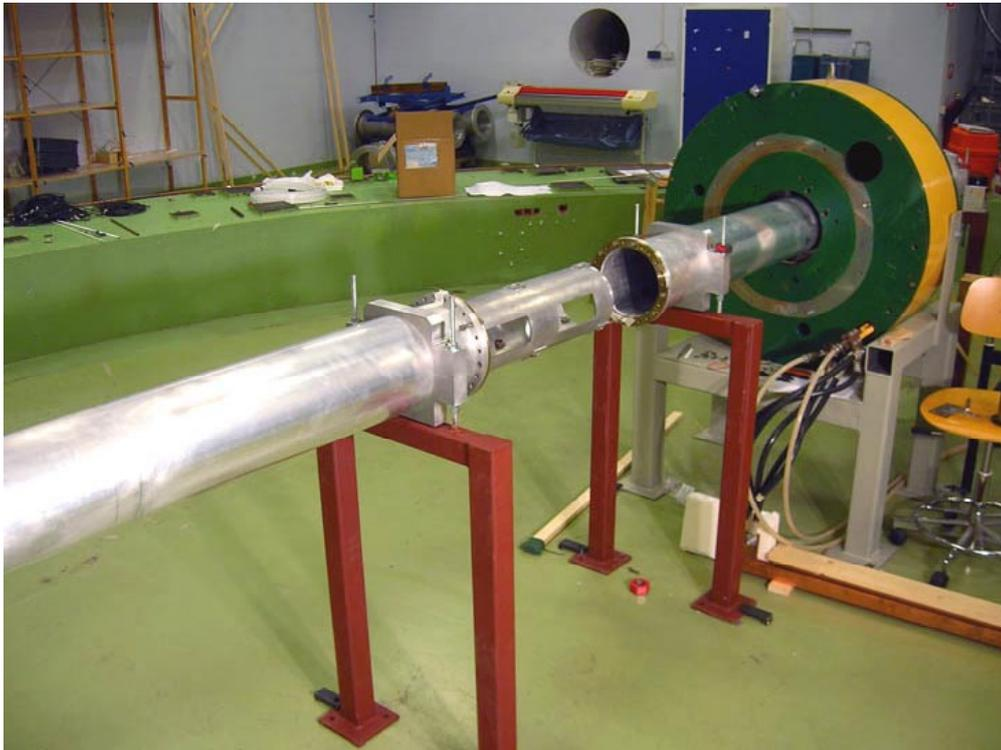
Figure 6-6: To the right in the figure, a setup for test of the sensor sensitivity. To the left and in the middle in the figure a setup for test of trolley movements. The trolley should be capable to bridge gaps in the ridges introduced by beam position measurement and scraper units. The trolley is drawn by a chain
