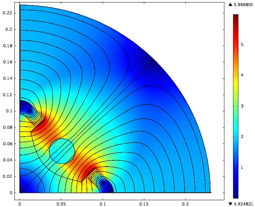
Figure 1. Calculated fields in the ICR arc quadrupole.
