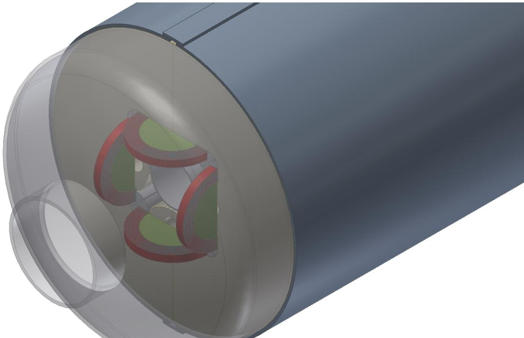
Figure 2. CAD design of quadrupole, showing winding ends, shell, and beam tube (quad not rotated to proper orientation in this view).
